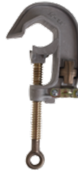
C6002282 Aluminum body, Serrated jaws, Bronze eyescrew with Acme threads Bronze pressure-type terminal
