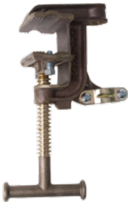
C6002231 Bronze body, Serrated jaws, Bronze T-handle with Acme threads, Drilled for 5/8-11 UNC threaded ferrule
