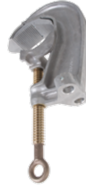
C6000375 Aluminum body, Serrated jaws, Bronze eyescrew with Acme threads, Dual drilled for 5/8"-11 UNC threaded ferrule
